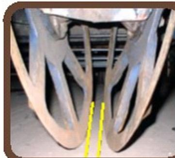
Before measuring your pinch points, take the time to spin the wheels and check for bent wheels and bad and/or loose bearings. If you find a problem, make sure you correct it before taking your measurements.
